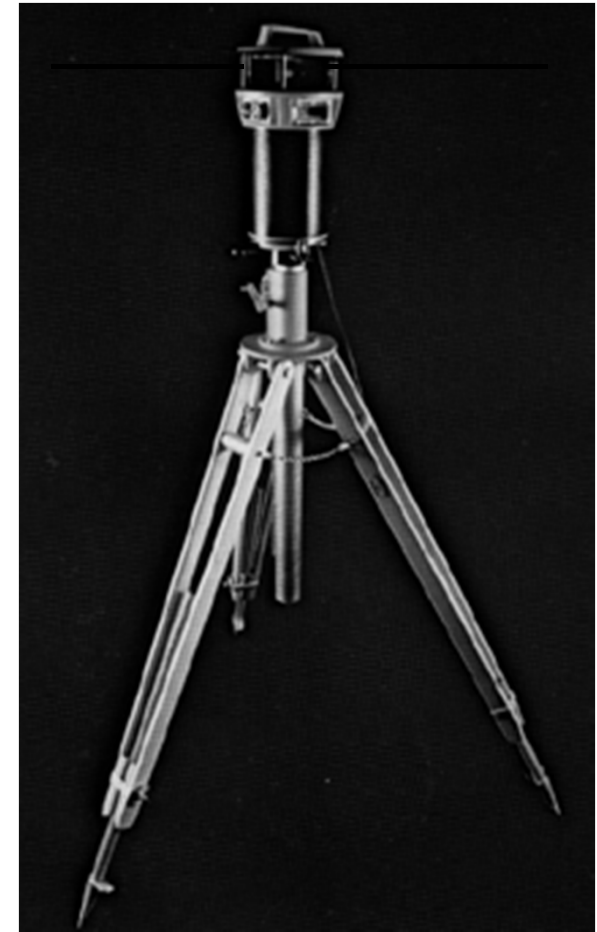
Typical laser level instrumentation tripod mounted
