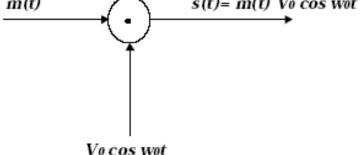
The product block allows, for example, achieving amplitude modulation of a carrier, obtaining as output a modulated signal s (t). Looking at the spectra, we have:
