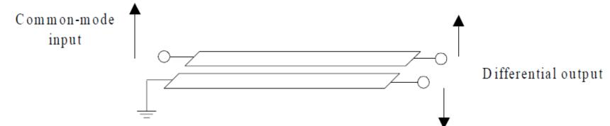
It is capable of bandwidths of over an octave, provided the coupling between the lines is high enough.
