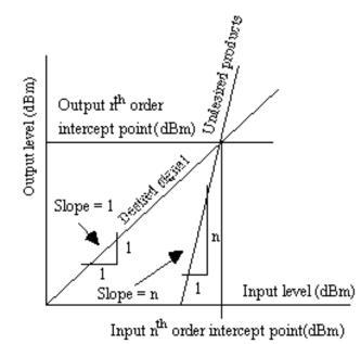
This output power level is the output intercept point, and equals the input intercept point minus conversion loss. defined as the difference in dB between the input and output S/N. The most common one is the third-order intercept point (TOI).
