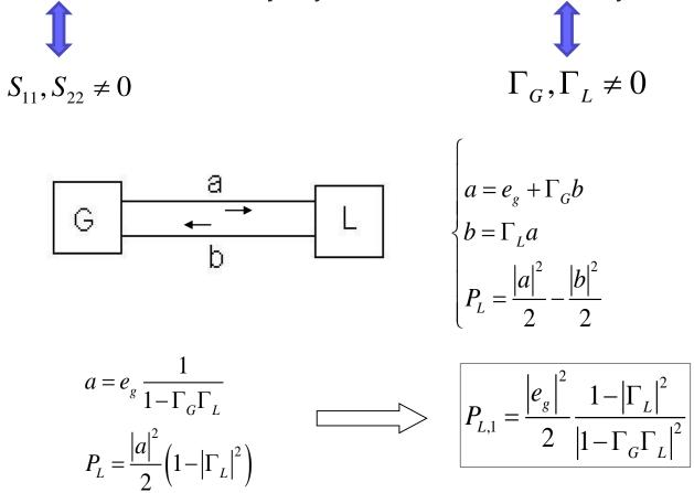
Now we insert the attenuator and calculate the resulting power received by the load. We have 4 equations: 1 at the source, 1 at the load, and 2 from the scattering matrix.
